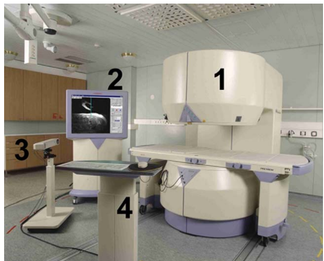
Fig. 2. Typical set up for low field IMRI facility: (1) the MR scanner, (2) the projector, (3) optical tracker camera, (4) user interface console (Panorama 0.23 TTM Philips Medical Systems MR-Technologies Finland, Vantaa, Finland).
